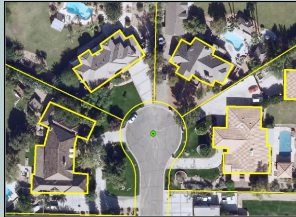
... are analytically co-registered to accurate ground survey control points
