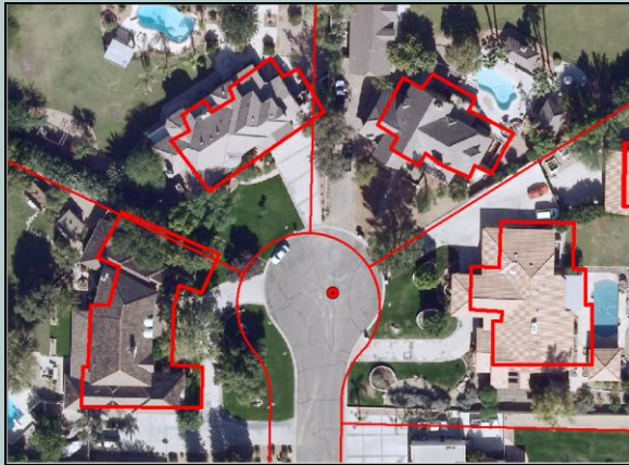
Misaligned GIS data, including property lines, building roof outlines, outdated survey points and background photography...
